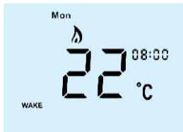
For 7 Day programming, only Mon is displayed in the day indicator field.
