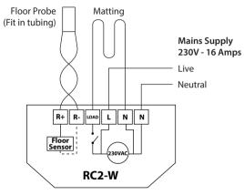
Mains supply must be fused correctly
