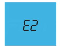
Check the sensor is correctly connected to the RT1 and - terminals at the rear of the thermostat (see wiring diagrams on page 26-28).
