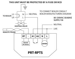
LS & LR ARE NORMALLY THE ROOM THERMOSTAT CONNECTIONS
