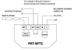
LS & LR ARE NORMALLY THE ROOM THERMOSTAT CONNECTIONS
