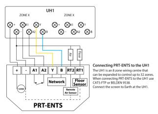
PRT-ENTS for use in wet area where floor temperature control or limiting is required.
