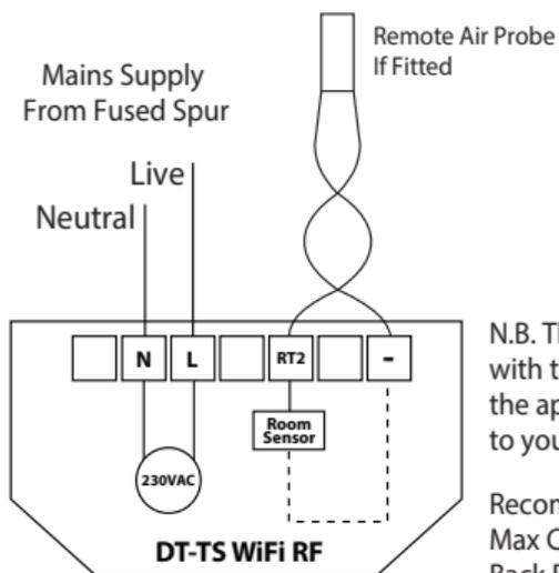
N.B. The DT-TS WiFi RF is designed to work with the RC1-W and the UH1-W. Please refer to the appropriate diagram for connections to your heating system.
