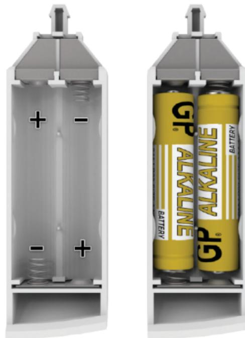
Insert the batteries in the empty battery holder, ensuring that each battery is orientated for the correct polarity + / - .
