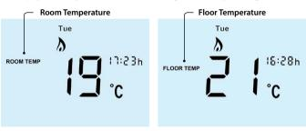
Note: Built in air sensor only MUST NOT be used to control electric underfloor heating. Floor sensor only or built in air & floor sensor together must be used.
