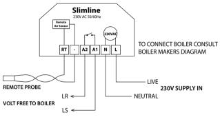
LS & LR ARE NORMALLY THE ROOM THERMOSTAT CONNECTIONS
