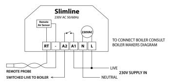
This product must only be installed by a qualified electrician and comply with local installation regulations.
