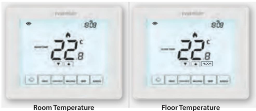
When the thermostat is set to use both the air & the floor sensor, the room temperature will be displayed by default.
