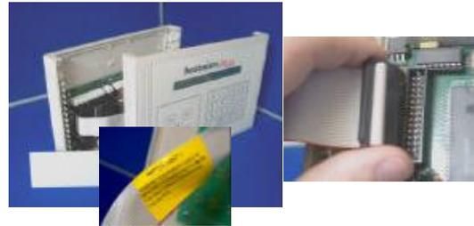
When you open the Heatmiser, remove the end panel first. You will notice a ribbon cable connecting the LCD board to the bottom circuit board.
