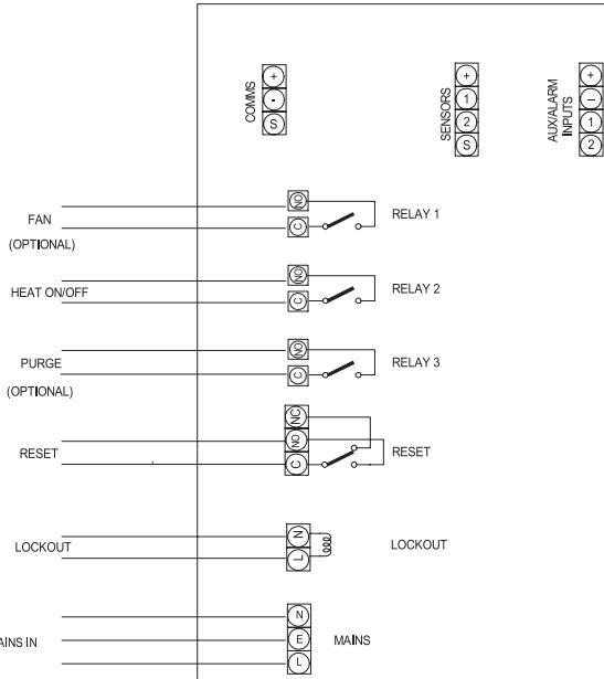
Beldon 8451 ( RS 360-649 ) Twin, Screened cable must be used when connecting the remote sensor and comms cables
