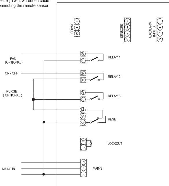
The reset command disconnects the live supply to the heater/s for a few seconds
