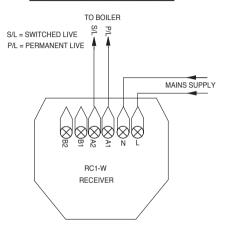
S/L AND P/L CONNECTIONS WILL VARY DEPENDING ON THE BOILER MODEL , BUT WOULD NORMALLY BE CONNECTED TO THE THERMOSTAT CONNECTIONS
