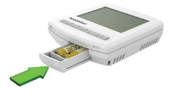
Push the battery holder back inside the thermostat until it is secured in its closed position.
