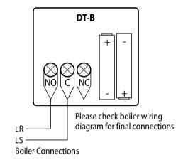
Note: LS & LR may be labelled differently but they are normally the boiler's room thermostat connections.
