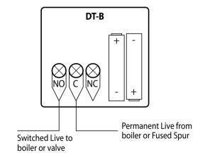
Note: When connecting to a valve, the valve auxiliary switch is used to enable the boiler.
