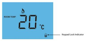
Note: The keypad lock indicator is only displayed when the lock is active.
